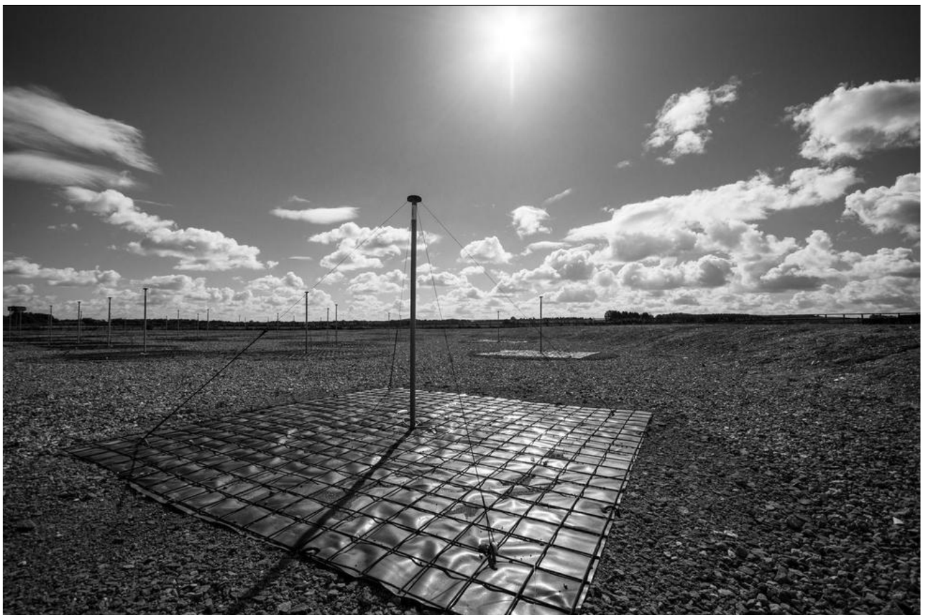
UK LOFAR antenna field - the European LOFAR system detects frequencies around 100MHz, roughly FM radio range. Thousands of simple dipole antennas, bit like old-style car radio aerials, feed into a centre in Groningen, Netherlands, where an IBM high-performance computer system combines and analyses the signals.
