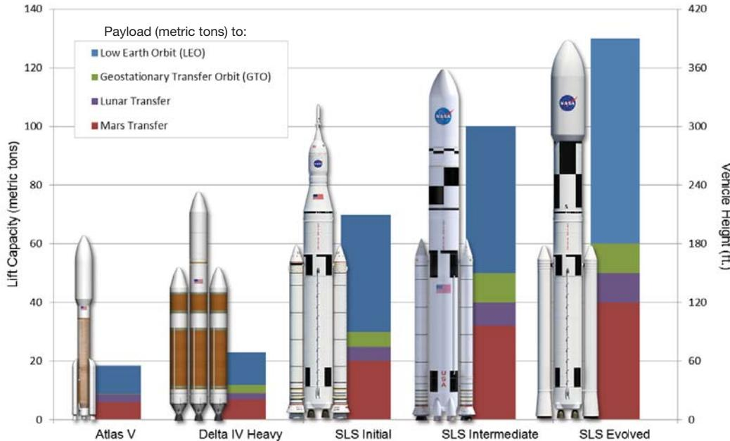
The vehicle's 5 m to 10 m fairing allows utilization of existing systems which reduces development risks, size limitations and costs. SLS lift capacity and superior performance shortens mission travel time.
